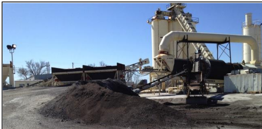
Figure A4.3. Plant RAP/RAS bins, screen, and conveyor belt entry into drum
