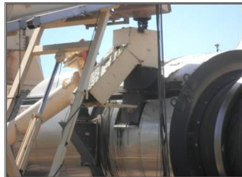
Figure B4.6. Adding RAS to drum
