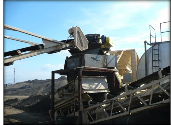
Figure C4.3. RAP gator recycling breaker
