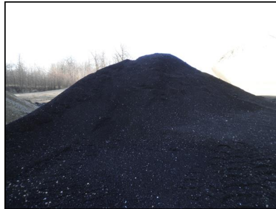
Figure E5.3. Recycled asphalt shingles (RAS) stockpile
